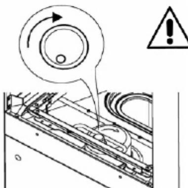
**WARNING:** In case of wrong direction of rotation, the mechanical to ensure the shift is ineffective.
